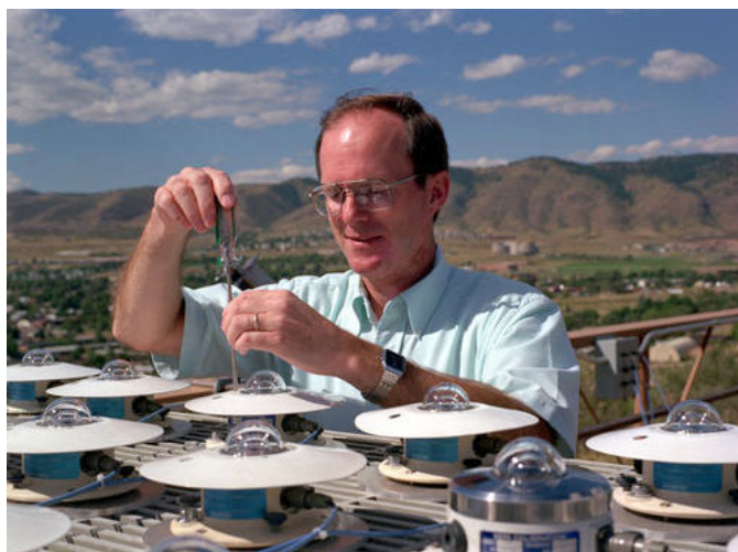
Figure 1. Calibration of pyranometers for solar irradiance measurements.
