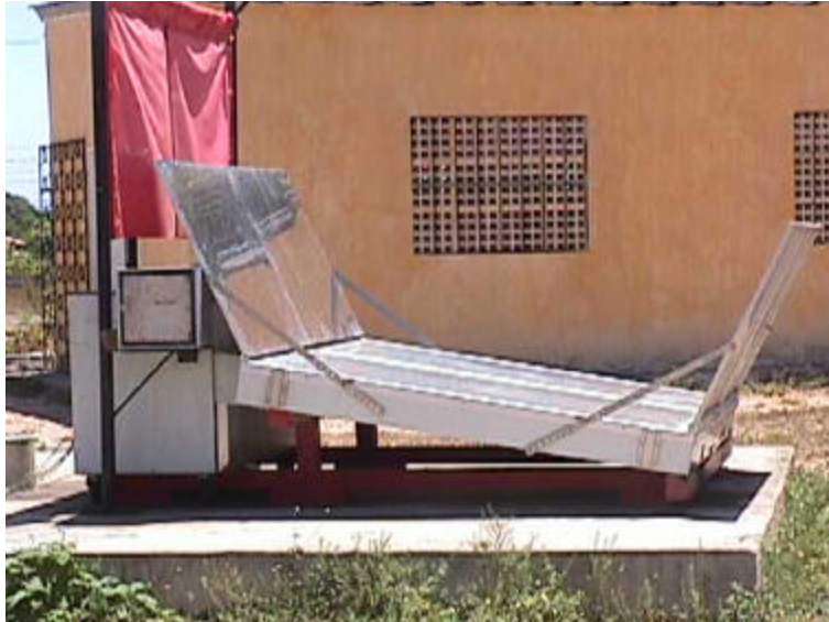
Picture 1. Photo of the solar cooker tested in Fortaleza - outdoors model with heat storage tank and oven.
