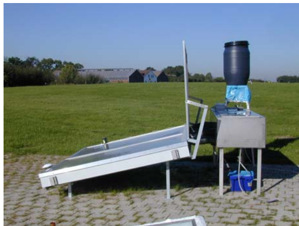
Figure 1. Photograph of the Solar Desalination Unit at the Solar-Institut Jülich in Germany.
