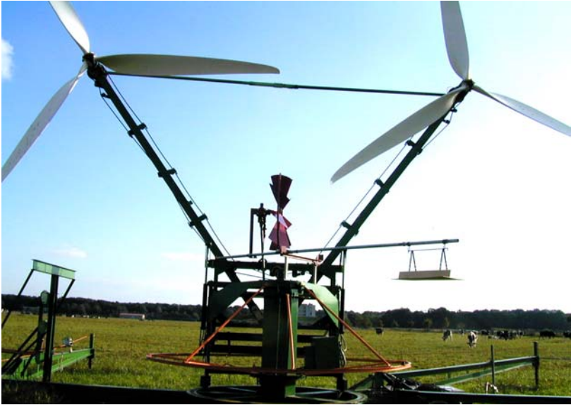
Figure 6: Photo of the MoWEC1 with Lee-wind wheel
