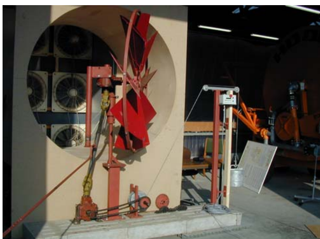
Figure 3, Figure 4: Lee-wind wheel inside the wind tunnel.
