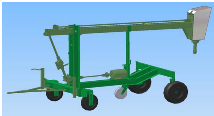
Figure 8: Working and transport position of the MoWEC2. Bivalent with diesel motor. For use energy application see Figure 1. Test in 2004. Street- und container transport.
