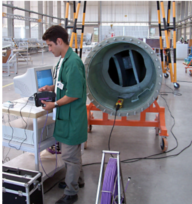
Fig. 3. Final check via an online-endoscope inside a blade for a 600 kW wind turbine at Wobben-Enercon in Pecém (35 km west of Fortaleza): Still Latin America's only manufacturer for large scale wind turbines.
