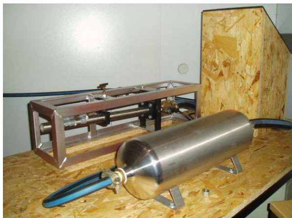
Fig. 5: Equipment ("ice ball gun") for carrying out impact resistance tests on solar collectors
