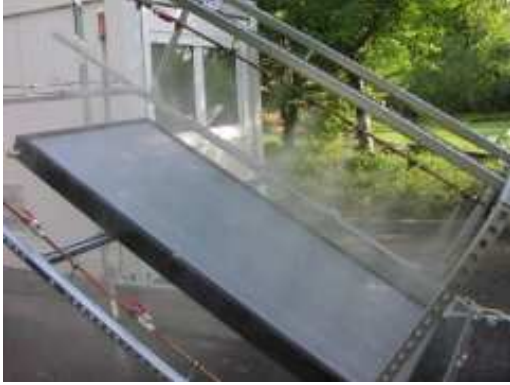
Fig. 3: Test facility for outdoor durability and reliability testing (here used for rain penetration test)
