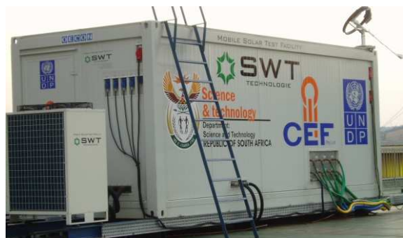
Fig. 6: Mobile, stand-alone test facility at SABS, South Africa
